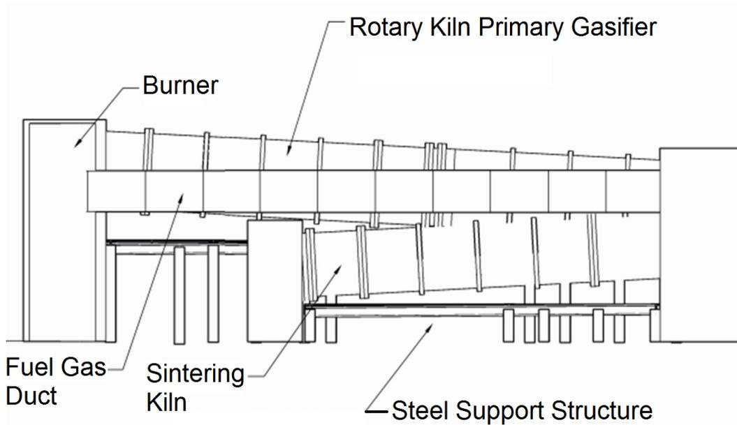
**Figure 5.** Elevation drawing of some of the core equipment for a 200 TPD system producing ordinary portland cement.
