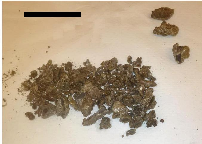
**Figure 4.** Clinker created from Turkish lignite and limestone. Scale bar represents 5 cm.
