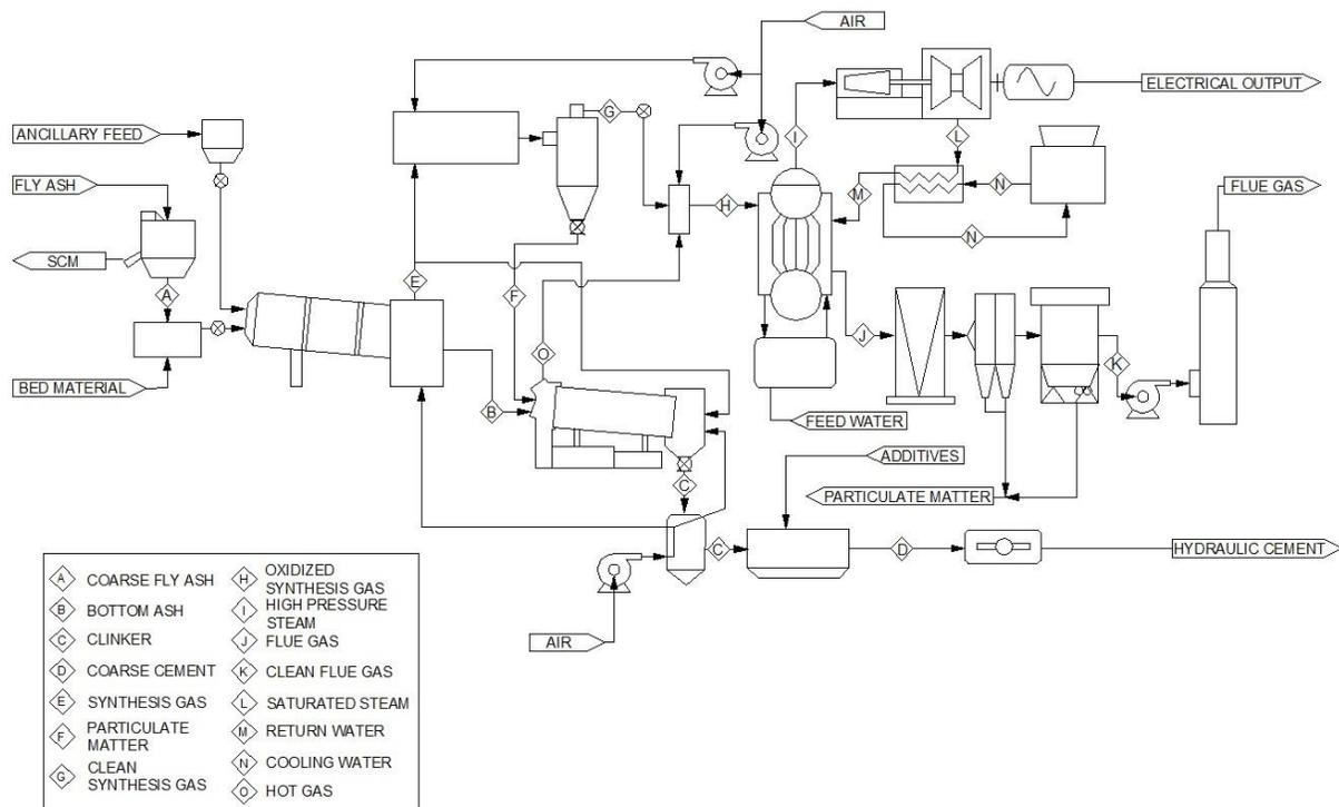
**Figure 1.** Process diagram showing the process feed system, first rotary kiln gasifier, the high temperature rotary kiln and clinker cooling and grinding equipment, as well as the fuel gas combustor, cyclone, boiler and steam power plant
