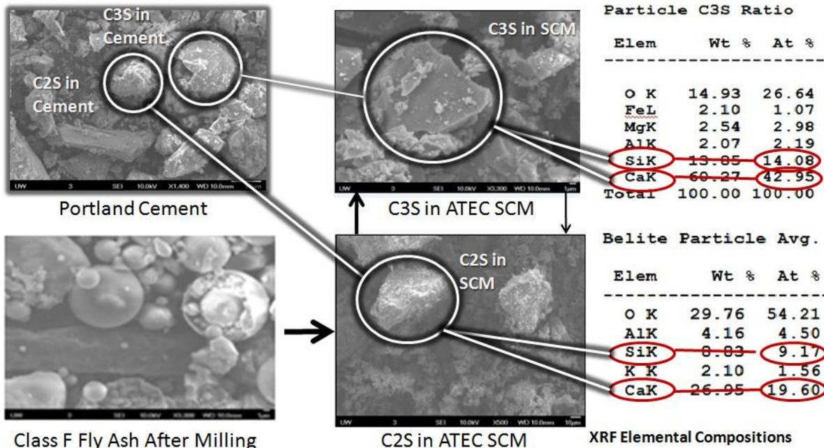
*ATEC cementitious material made from Kingston, TN ponded fly ash*
