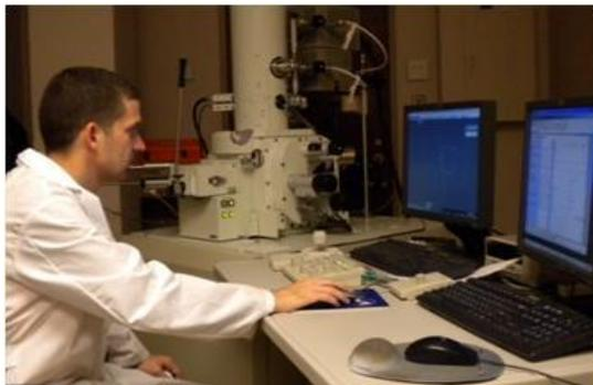
**Figure 3.** Scanning electron microscope with EDAX XRF for determination of particle elemental compositions
