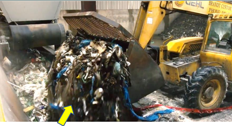
No shredding is required for run of the dump waste.
