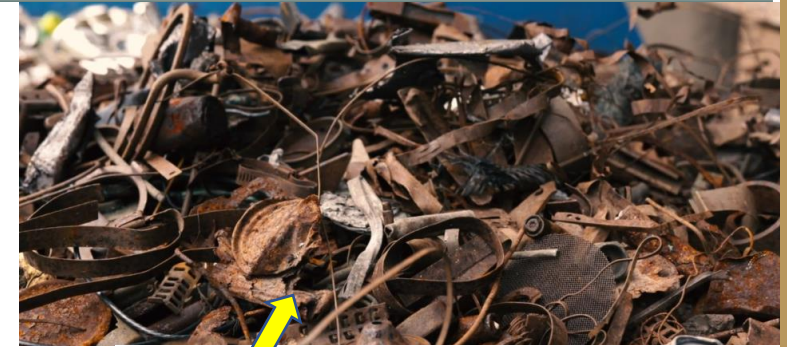
Steel scrap recovered from unsorted waste after gasification
