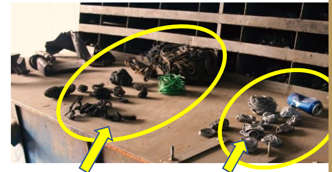
Ferrous metals and aluminum can be recovered after combustible components are gasified
