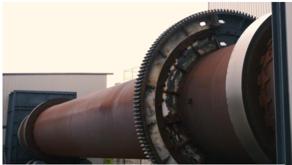
Rotary kiln operating on run of the dump waste.
